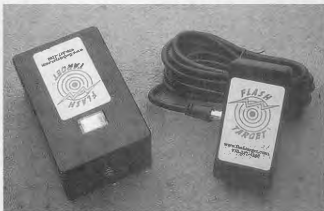
Flash Target mounts on the rear of any steel target, to emit a bright strobe flash when the steel is hit.
